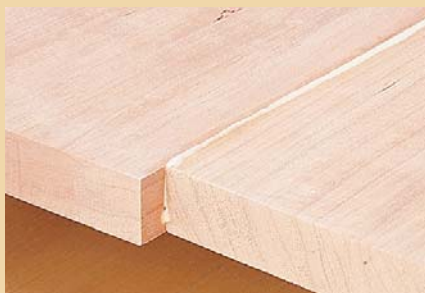
▲ How much pressure? Apply clamping pressure until an even bead of glue forms along the joint line.
