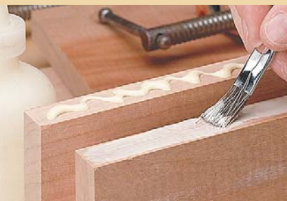
▲ How much glue? A strong joint needs a thin, even layer of glue. Spread the glue with a brush or piece of scrap.
