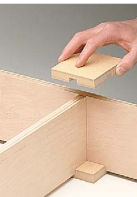
▲ These assembly blocks help hold parts of a case until the clamps can be positioned. Just cut a pair of intersecting dados in pieces of scrap.
