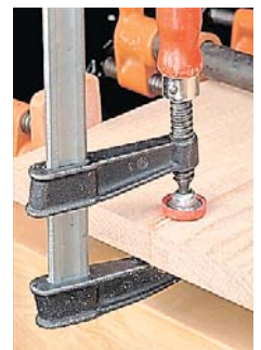
▲ Tightening a clamp across the end of a joint line draws the surfaces of the boards flush.
