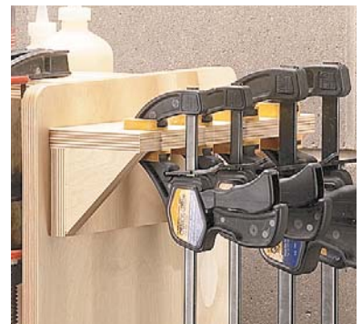
▲ Pistol-grip clamps can be cinched down on a rack, ready to grab and be put to work.
